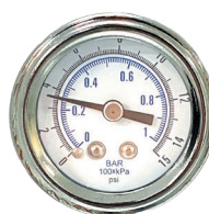
Flow regulator valve with pressure gauge displaying the actual He pressure in psi and bar.
