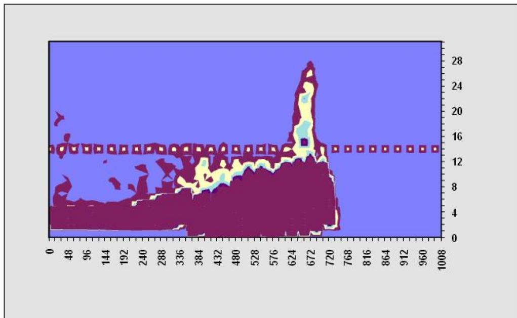
Figures above show example results of 60 CPM of Americium with 100 000 CPM of Thallium. The results show the excellent separation capabilities with virtually 0% misclassification.
