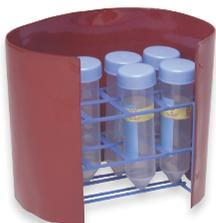
Lead sheets are 0.09" (2.2 mm) thick and provide effective shielding from <sup>125</sup>I.
