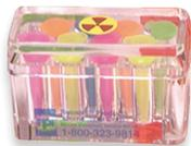
Clear acrylic for maximum viewing of sample tubes, the shield is 0.4" (10 mm) thick and holds 24 x 0.05 - 0.07 fl oz (1.5 - 2.0 ml) and 15 x 0.02 fl oz (0.5 ml) tubes.
