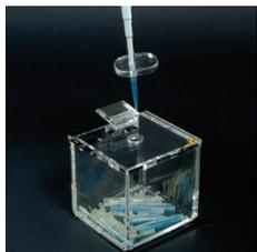
Can be used in conjunction with drawstring bags to give a convenient and visible area to dispose of radioactively contaminated tips.
