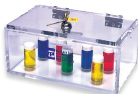
Store in a freezer (to  $-70^{\circ}\text{C}$ ) or add crushed ice to keep samples cold for bench top use.
