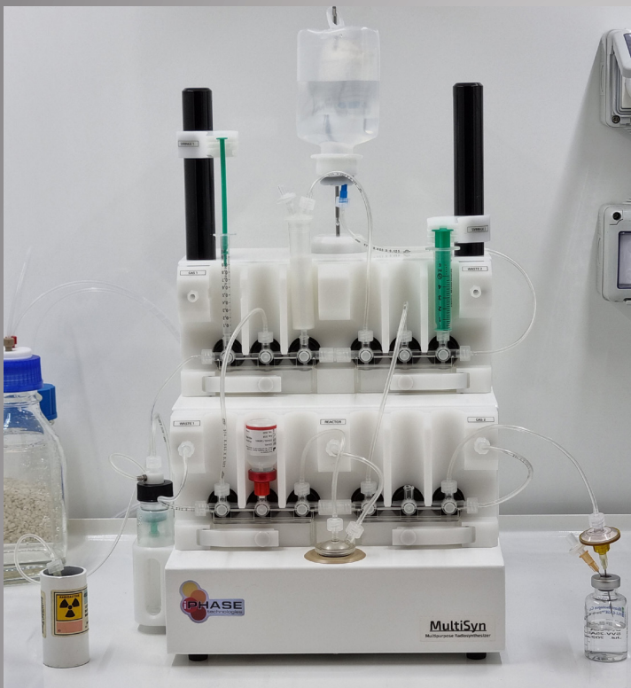
Setup for ^{89}\text{Zr} radiolabelling.
