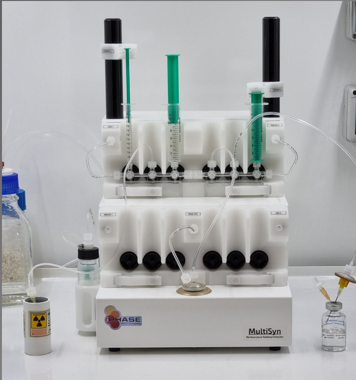
Setup for ^{177}\text{Lu} -PSMA & ^{177}\text{Lu} -DOTATATE radiolabelling.
