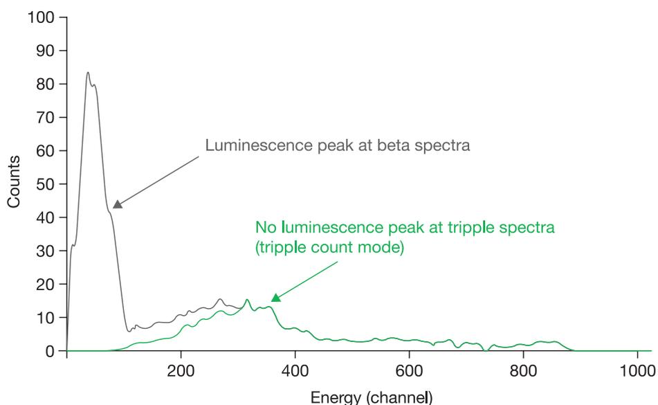
**Figure 3. Direct detection of bio-oil fraction with triple count mode.** Bio-oil samples with variable degrees of color luminescence interference were analyzed using direct measurement on Hidex 300 SL. 10ml oil-samples were mixed with 10ml MaxiLight cocktail, and the samples were counted for 100min (counting window 110–580). (A) A luminescence interference peak appeared in double counts (black spectra), but did not interfere when triple counting mode was utilized (green spectra).
