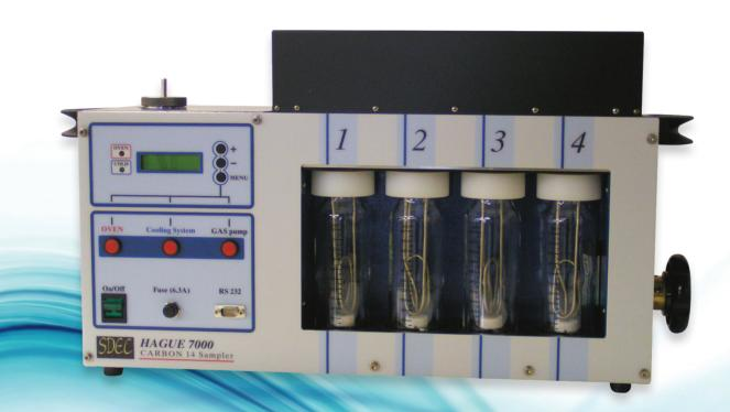
The Hague 7000 <sup>14</sup>C sampler from SDEC is the perfect instrument for measuring low levels of <sup>14</sup>C in air.
