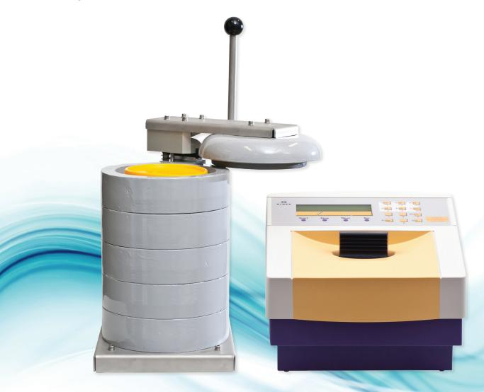
Triathler Becquerel Finder is optimised for detection of radioactive isotopes in the event of a nuclear emergency in food. The instrument is equipped with an external NaI detector with an enlarged lead shield, which facilitates the use of Marinelli beakers with total sample volume of up to 1L. This enables rapid detection of I-131, Cs-134 and Cs-137 in foodstuff, water and milk.
