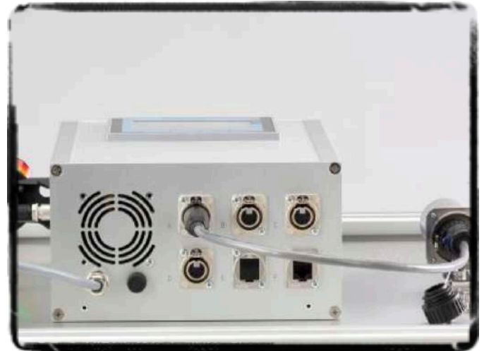
Free to choose communication ports. Ethernet & USB output for relays and detector ports.
