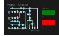
Animated flow-path diagram shows instrument status in real-time and allows sample flow to be tracked.
