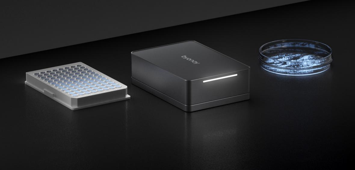
Using 96 highly sensitive silicon photomultipliers, Luminescence 96 is an entirely new type of luminometer.
