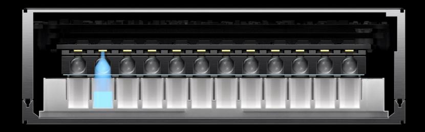
With Luminescence 96, every millimeter counts. By bringing the microplate within a 10th of a millimeter of the detector, cross-talk is, at  $< 0.7 \times 10^{-6}$ , practically eliminated.
