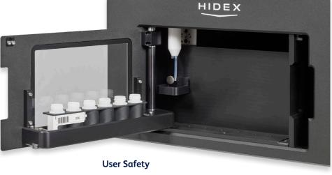
The user can specify a timed flow of cooling air past the ladles along with a specified time for the safety interlock on the ladle cover to protect the user from contact with the hot ladles following the oxidisation process.
