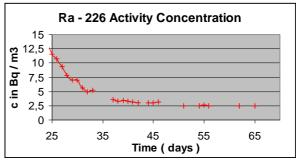
Fig.1: background corrected decay curve
