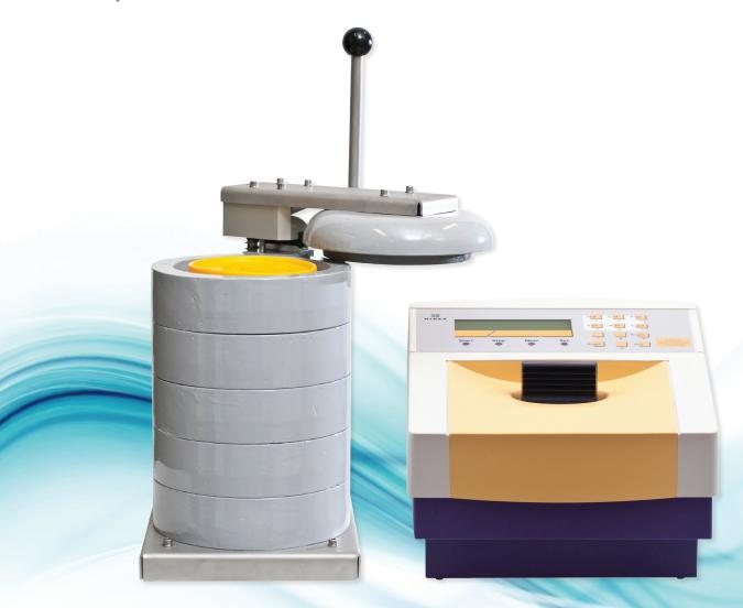
Triathler Becquerel Finder is optimized for detection of radioactive isotopes in the event of a nuclear emergency in food. The instrument is equipped with an external NaI detector with an enlarged lead shield, which facilitates the use of Marinelli beakers with total sample volume of up to 1L. This enables rapid detection of I-131, Cs-134 and Cs-137 in foodstuff, water and milk.
