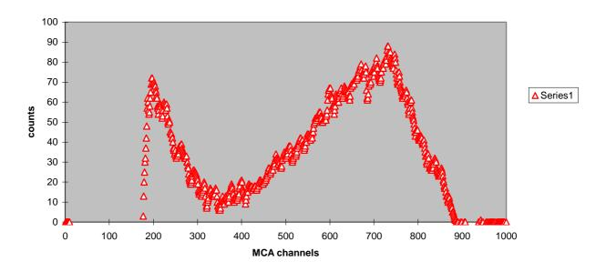
The figure shows an alpha spectrum, of an wipe test with Pu-239, measured over a time of 10 hours. The alpha signal clearly is visible.
