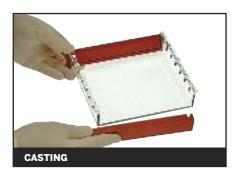
'Plug-and-Go' casting – moulded casting dams clip easily onto the ends of the gel tray for rapid external casting, allowing the multiSUB™ unit to remain in use for gel running. Casting is as simple as 1, 2, 3... place one dam onto the lab bench facing upwards and insert the tray into the groove in the dam and repeat with the second dam at the other end. The tray is now sealed and may be placed on flat bench space or gel levelling table in readiness for leak proof gel-casting.
