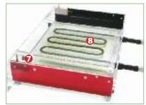
Replacement IEF Tank, CSL-IEFTANK (Tank/Electrode Only, No Cooling Platform)
